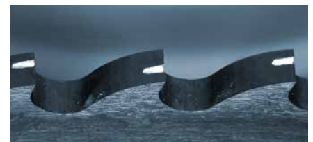
Curved back teeth with chip breaker grooves
