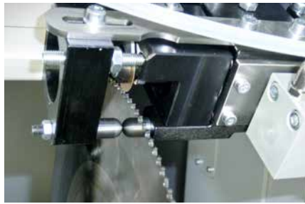
Attachment to grind in chip breaker grooves ▶▶ 2
