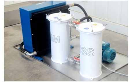
External HSS- and carbide filter with coolant chiller unit
