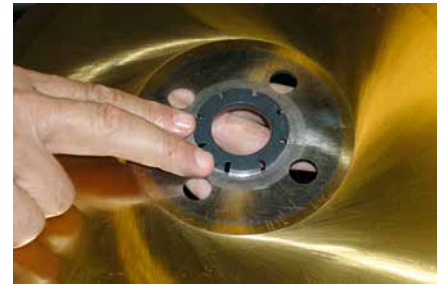
Reduction ring to create a bore size suitable to the arbor in use
