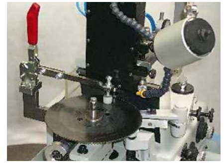
Fast saw blade tensioning system
