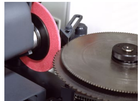
Sharpening by means of master index plate, recutting or cutting teeth into blanks
