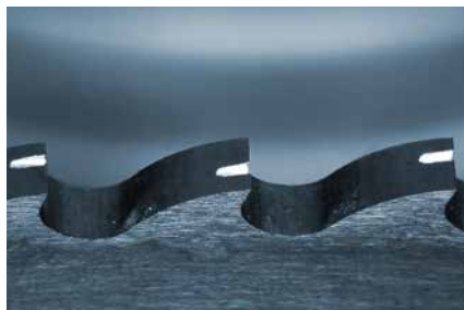
Curved back teeth with chip breaker grooves
