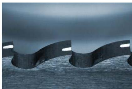
Curved back teeth with chip breaker grooves
