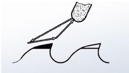
Movement of the grinding head on Bi-Metal band saw
