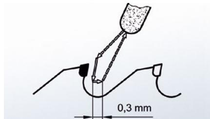
Movement of the grinding head on carbide-tipped band saws
