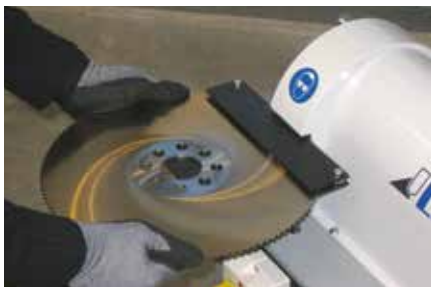
Saw blade chip/burr removal
