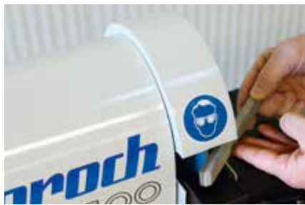
Dressing of CBN grinding wheel
