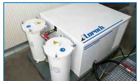
Polar chiller with HSS and carbide filter
