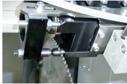
Attachment to grind in chip breaker grooves VIDEO 2
