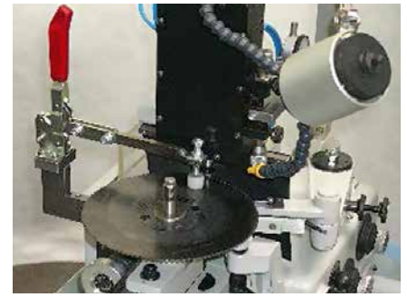
Fast saw blade tensioning system
