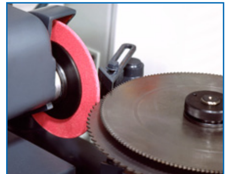
Sharpening by means of master index plate, recutting or cutting teeth into blanks
