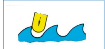
1. The grinding wheel moves into the tooth and contacts slightly the tooth face
